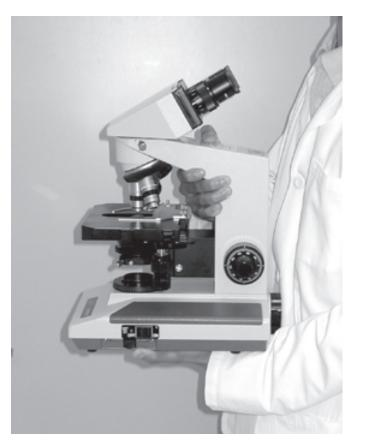
The condenser can be lowered or raised by an adjustment knob. Lowering the condenser decreases the amount of light that reaches the object. This is usually a disadvantage in microbiological work. It is best to keep the condenser fully raised and to adjust light intensity with the iris diaphragm.
