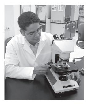
Turn the adjustment knobs *slowly* and *gently*, as you pay attention to the relative positions of the objective and object. Avoid bringing the objective *down* with the fine adjustment while viewing, because even this slight motion may force the lens against the object. Bring the lens safely down first with the coarse knob; then, while looking through the ocular, turn the fine knob to *raise* the lens until you have a clear view of the subject.
